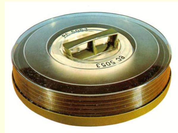
7.25 MB Disk Drive Unit US 5052 with removable disk pack US 5053 (1971)
